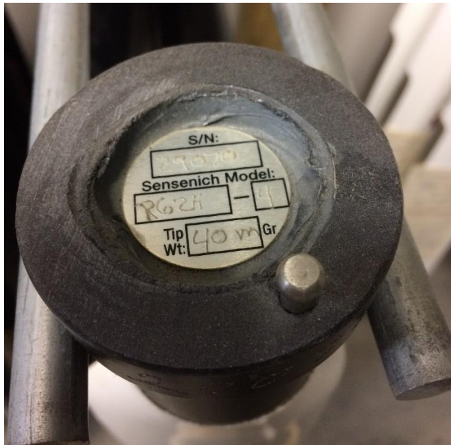
Figure 2: Shank plug with added shank weights. (Note: Plug appears to be relatively shallow, approximately ¼" or less with thickened resin underneath the metal data tag.)
