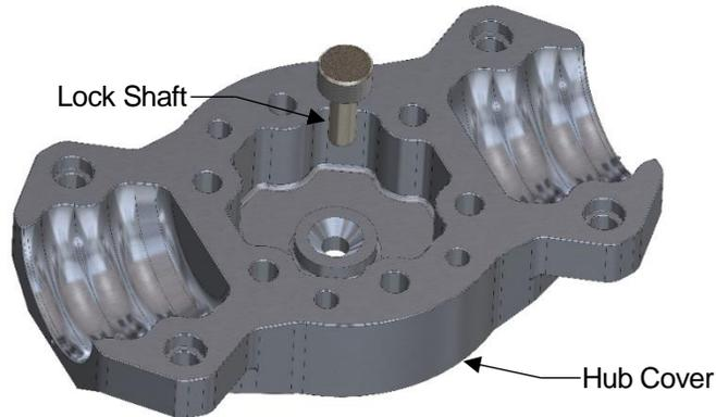
2. After finalizing blade pitch, slide the lock plate on top of the cover half and protruding lock shaft, making sure the lock plate indexing cutouts match up to the indexing boss on the hub face, shown below
