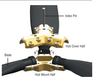
Sensenich's new **Index Pin Pitch System** also lets its user select from a variety of pitches and set a specific pitch. The index pin is placed in the hub, and the blade pins are set against it. To change the pitch, you simply loosen the clamp bolts, place the new index pin in the hub, set the blade pins against the index pin, torque the clamp bolts and remove the index pin.
