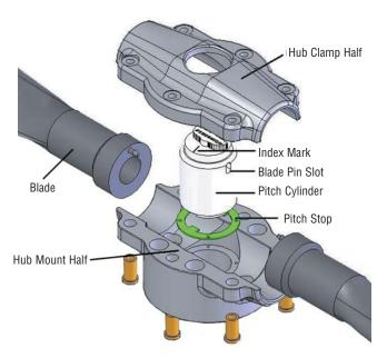
Sensenich's new **Pitch Cylinder Hub System** allows its users to set a broad range of pitches, using the system's index mark as a reference point when making adjustments. They adjust 16 degrees in pitch, affording maximum performance within an efficient aerodynamic envelope. The blade pins lock into the blade pin slot of the pitch cartridge, allowing the blades to move back and forth in tandem for ease of setting pitch.
