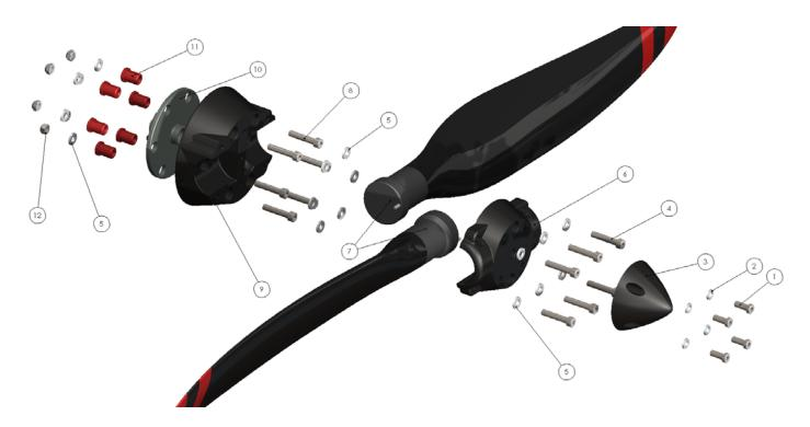
FIGURE 1. 2A2V5 PROPELLER ASSEMBLY
