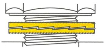
FIGURE 3. NORD-LOCK LOCK WASHER
