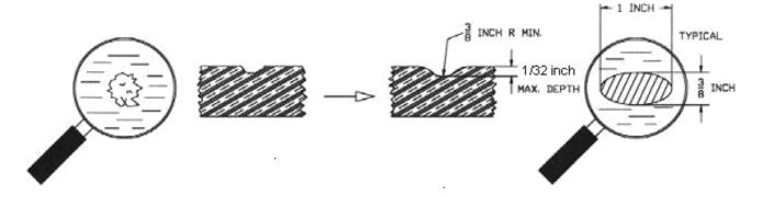
FIGURE 6. MINOR HUB REPAIR LIMTS
