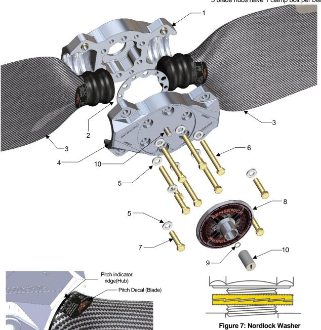
Figure 6: Pitch Setting Detail
