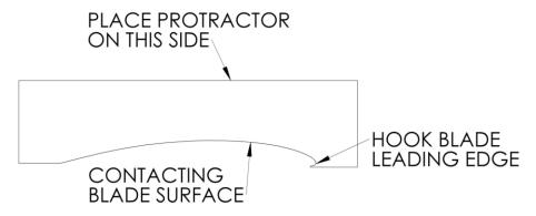
Figure 5: Sensenich 75% Full Contact Template Example
