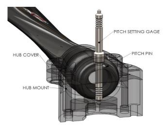
Figure 9: Pitch Setting Gage Detail
