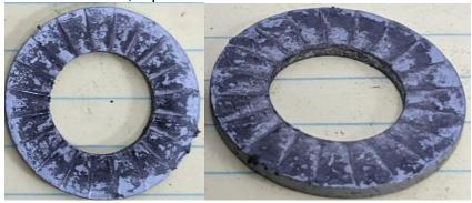
(c) Washer wear equivalent to or beyond the illustrations of **SECTION 1G1(c)** is considered high use with approximately 50 installations. Minimal silver coating exists. Significant darkening and rounding along the vertical edges. Nord-lock must be retired. If any doubt exists on washer condition, replace washers.
