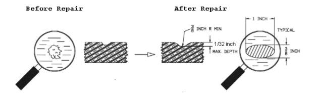
Figure 11: Minor Hub Repair Limits
