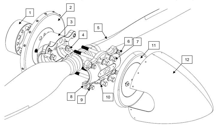
**Figure 1: Propeller Assembly**A-1608 and Airfoil Template not included in Figure 1.
