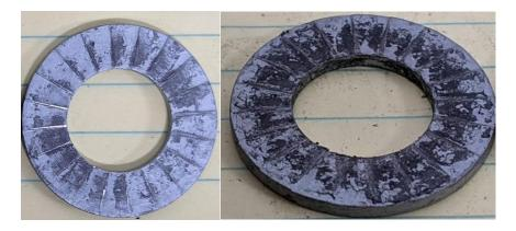
(b) Washer wear equivalent to the illustrations of **SECTION 1G1b** is considered medium use with approximately 10-40 installations. Minimal silver coating exists around the outer edges of the ramped faces. Re-use of Nord-lock is acceptable. If any doubt exists on washer condition, replace washers.
