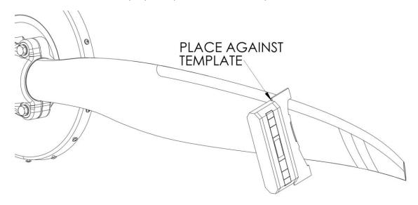
Figure 8: Template and Digital Level/Protractor Positioned on Blade.
