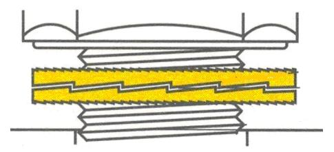
Figure 2: Nord-Lock Lock Washer
