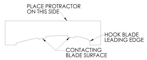
Figure 4: Sensenich 75% Partial Contact Template Example
