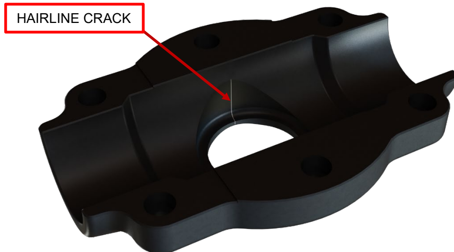
Figure 4. Cracks start near pitch marks and grow outwards. Inspection inside the hub cover is required.
