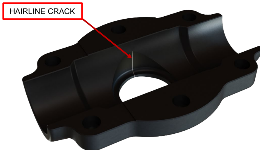
Figure 1. Cracks start near pitch marks and grow outwards.
